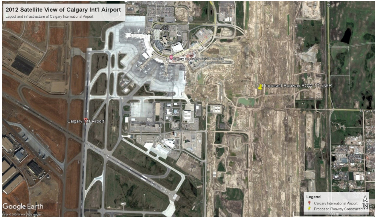
Figure 1. Historical satellite view of Calgary International Airport in the year 2012 from Google Earth Pro. Map shows ongoing construction of the 14,000 feet (4,270m) Runway 17L-35R
